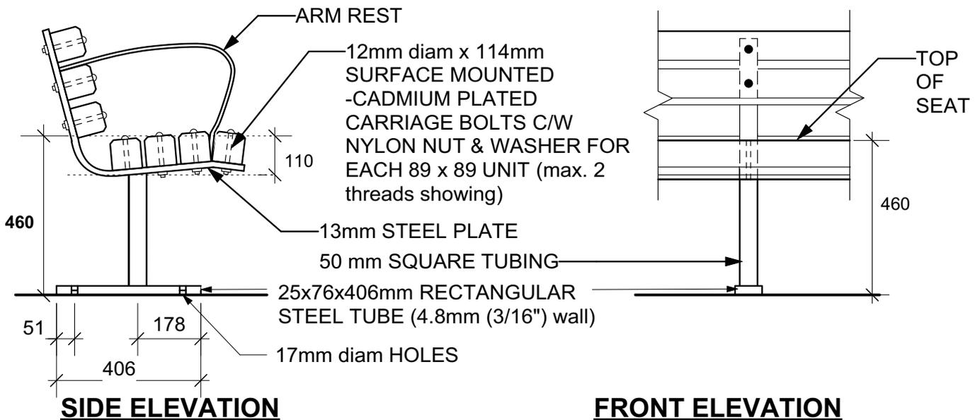
DIMENSIONS SHOWN ARE IN MILLIMETRES UNLESS OTHERWISE SPECIFIED
